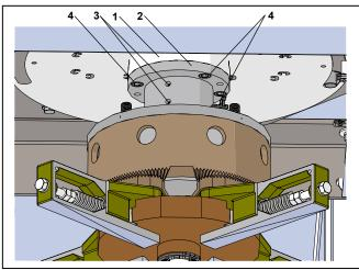
Fig. 22.1.6 Slip ring and bookfold lock coil wiring
