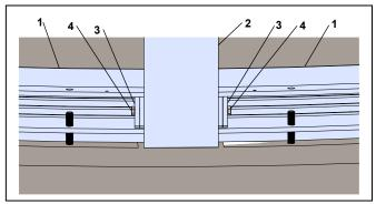
Fig. 19.3.2 Bottom rail attached to end walls
