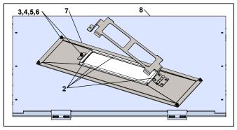
Fig. 20.3.10 Intenta sensor placed on Intenta sensor bracket
