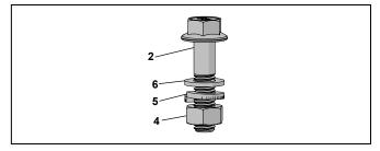
Fig. 20.3.2 K9 drive M8 x 35 flanged hex head screw and turnbuckle assembly
