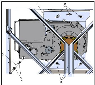
Fig. 23.5.5 Wing assembly overhead view: wing aligned with end wall secondary closing edge
