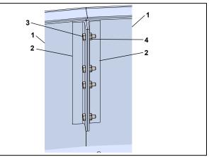
Fig. 13.2.5 Canopy soffit fasteners
