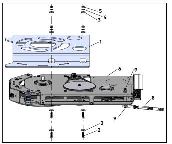
Table 7.3.3 Assembly, drive, K9 unit and mounting bracket RS6086
