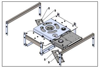
Fig. 7.5.3 Kit, K9 drive assembly, 1 Intenta sensor, exploded view
