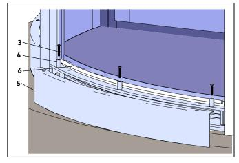
Fig. 25.5.3 Bottom rail cover installed
