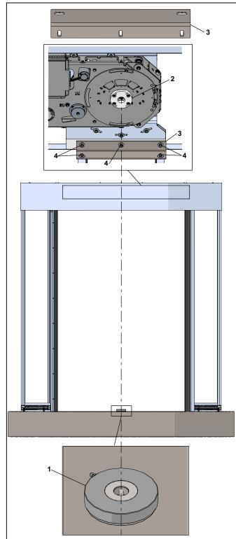
Table 20.1.1 Floor pivot bearing and K9 drive coupling
