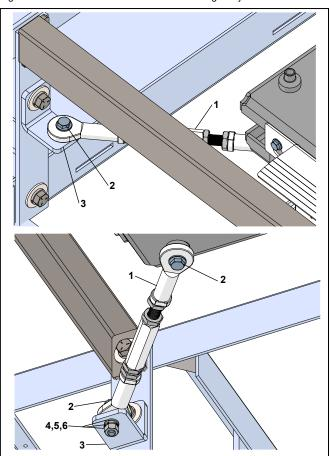
Table 20.3.1 K9 turnbuckle assembly mounting hardware
