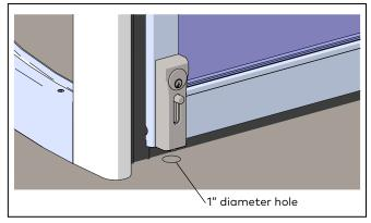
Fig. 24.1.4 Floor strike installed
