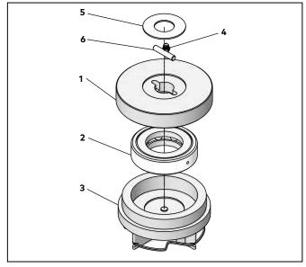
Fig. 11.6.2 Floor bearing assembly installed in floor
