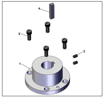
Fig. 21.2.2 RK6013 collar assembly above splined shaft
