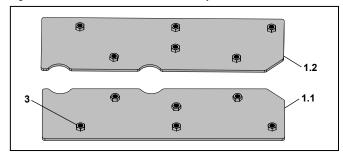
Fig. 15.2.2 Side mount weldment fasteners
