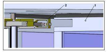
Fig. 23.4.3 Wing installation on hanger
