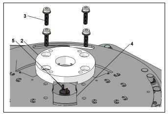
Fig. 12.1.4 K9 main drive adapter coupling installed
