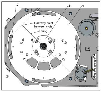
20.4.1 This procedure will align the K9 drive locking disc locking bolts with the end wall.
