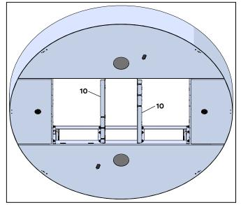
Fig. 13.3.4 Cover plate support bracket and fasteners
