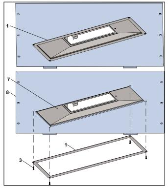
Fig. 20.3.9 Intenta sensor bracket installed on cover plate
