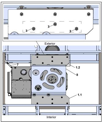
Fig. 15.4.4 K9 drive assembly mounting, bottom view
