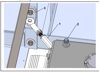
Fig. 20.3.3 K9 drive turnbuckle fastened to angle adjustment bracket
