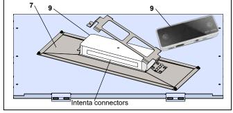
Fig. 20.2.11 Sensor cover secured to sensor bracket
