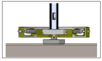
Fig. 22.1.2 K9 main drive adapter set screws loosened
