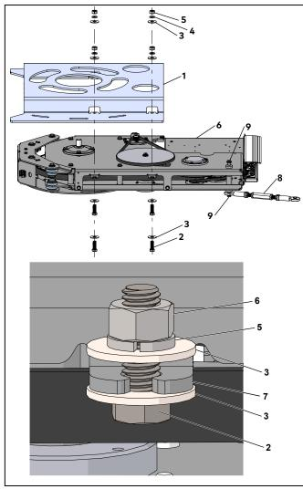
Table 12.2.1 Assembly, drive, K9 unit and mounting bracket RS6086
